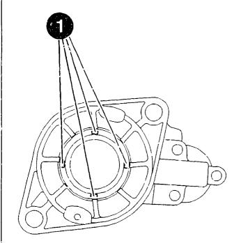
Checking drive-end bearing
